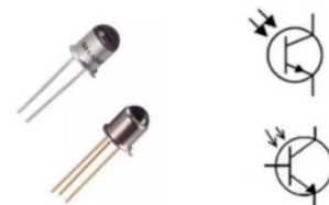
Fig. 2. The shape and symbol of the phototransistor sensor
