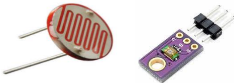
Fig. 5. (a). LDR sensor (b). Phototransistor sensors
