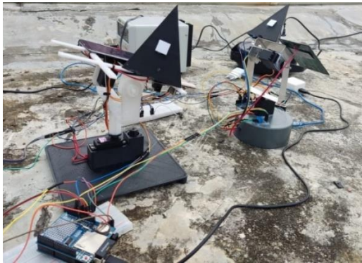
Fig. 11. Prototype Sun Tracker dual-axis based sensor
